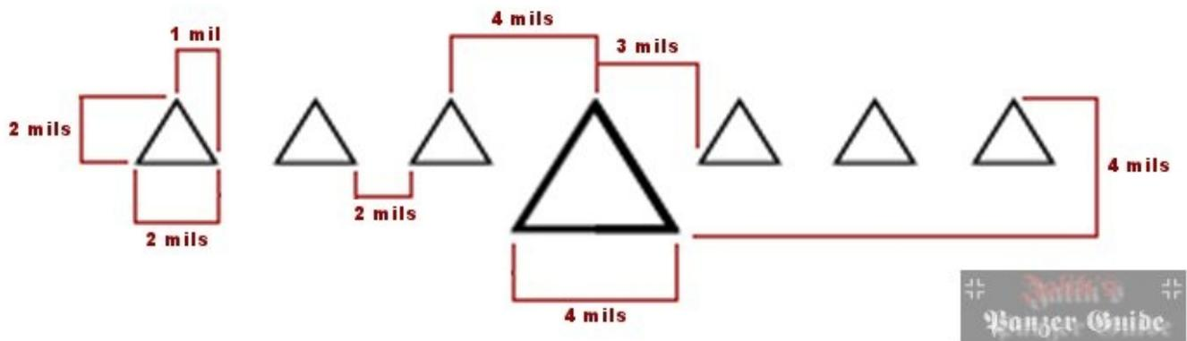
If a tank seen from the side fits between the upper edge of the main triangle and the upper edge of one of the neighboring small triangles it's "4 mils long". If a tank seen from the front fits into one of the small triangles it's "2 mils wide".
